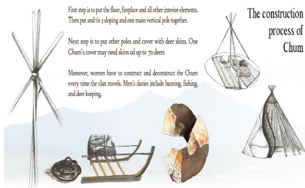
Figure 1. Construction process (Developed by Author).
